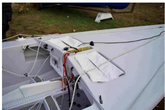
foto 3 – Particular of the mast guide and of the spinnaker slots.
